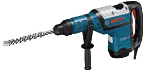
GBH 8/45 D Kırıcı-Delici Matkap 952.00 € 1500 watt, 45 mm çap, 8.2 kg, 12.5 Joule, SDS Max
